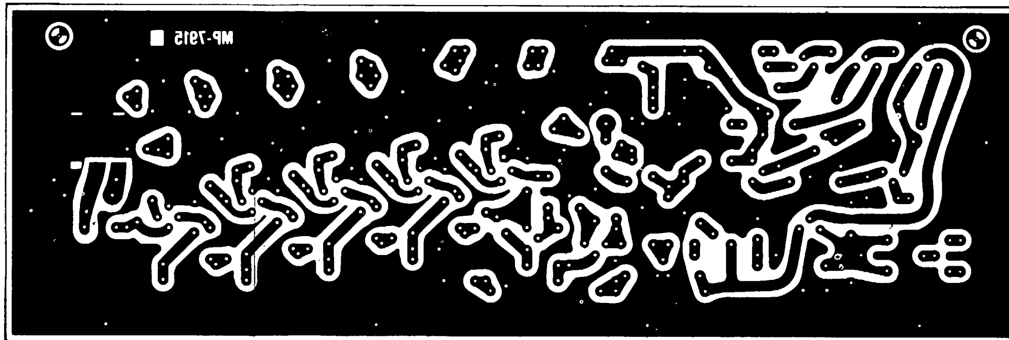
B. WIRING ON BACK OF BOARD A4 (VIEWED THROUGH FRONT)
